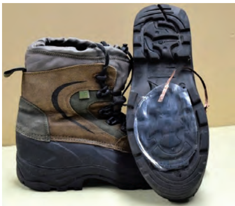
The first-of-its-kind nanogenerator called snow TENG, attached to a hiking shoe.
