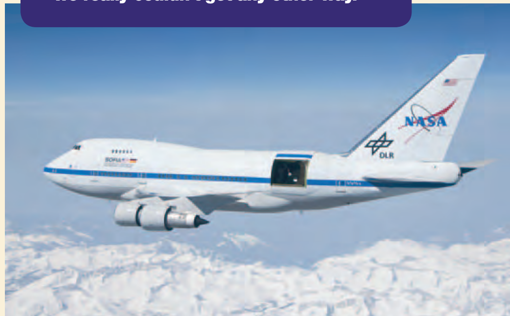
SOFIA, a modified 747 jetliner, houses an observatory in its mid-section that, when flying at 45,000 feet, will provide the clearest view yet of the center of the Milky Way.
