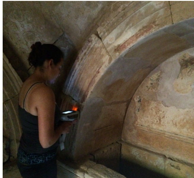
UCLA student in Cyprus examining Roman tomb painting using portable XRF
